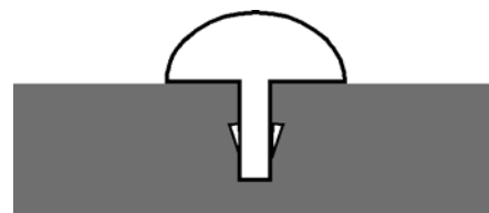
Side view of a fret in its slot
